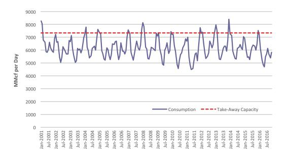
Figure SR-2.3. Average Daily Gas Consumption By Month vs. Pipeline Take-Away Capacity (MMcfd - millions of standard cubic feet per day).
