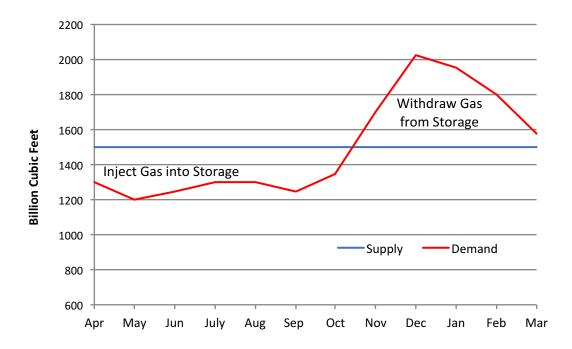
Figure SR-2.2. Example: Using Storage to Manage Variable Demand Against Flat Supply.
