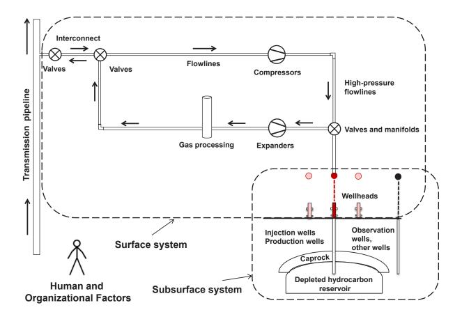
Figure SR-1.2. Simplified schematic of the main components of underground gas storage facilities in California, showing examples of engineered surface components and the wells and geologic features comprising the subsurface system. Human and organizational factors play a critical role in control of both surface and subsurface systems.
