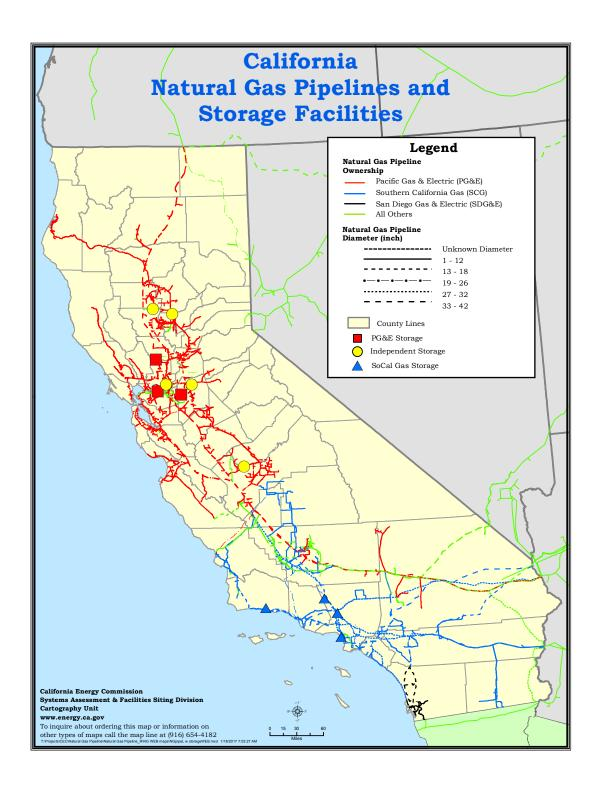
Figure SR-2.1. General Layout of California High Pressure Pipeline and Storage Facilities.
