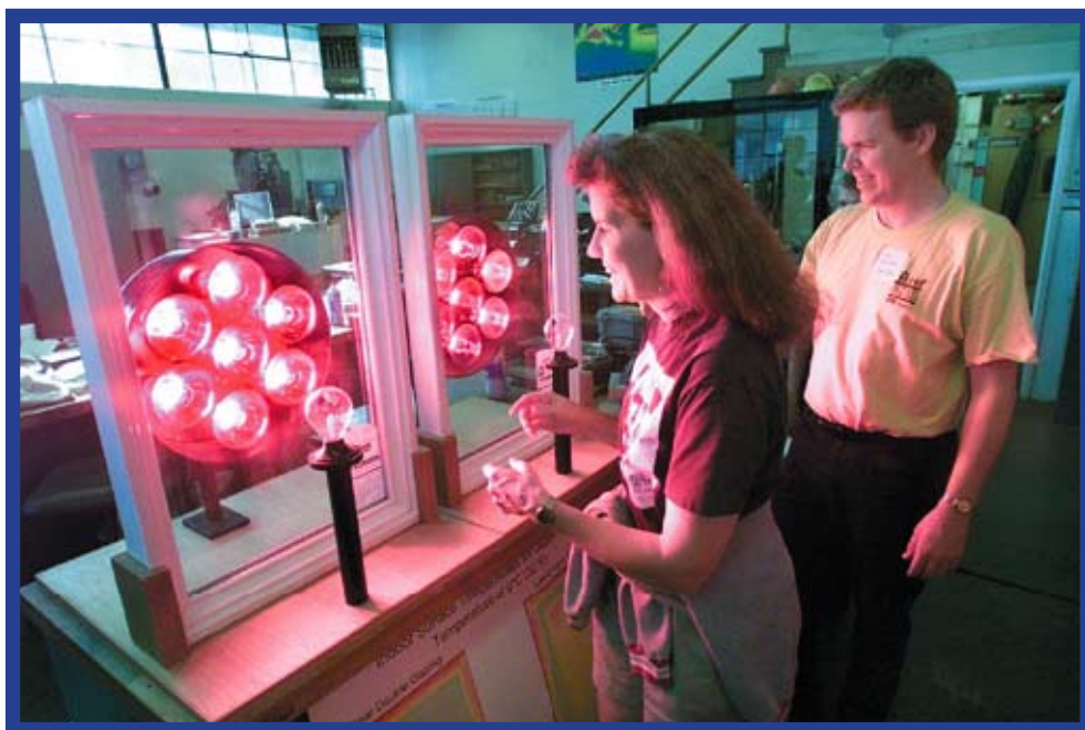
Windows heat test at Berkeley Lab, comparing the heat flow through a standard window and that through a dual-pane window with low-emissivity coatings.
