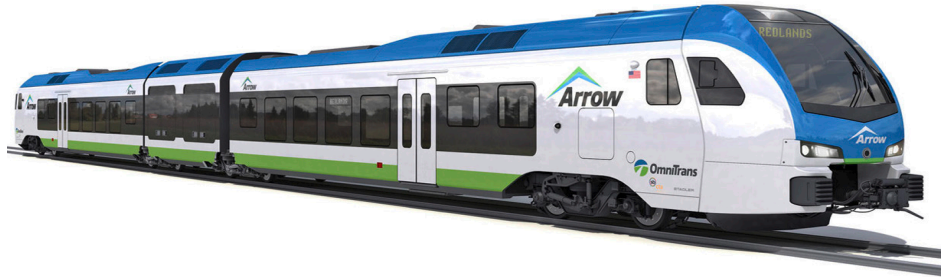
Figure: San Bernardino County Transit Authority (SBCTA) is working to develop the nation's first hydrogen-powered passenger train. Sandia National Laboratories has been supporting SBCTA through discussions on safety standards for the train and the necessary supporting infrastructure (e.g., refueling and maintenance facilities). (SBCTA)
