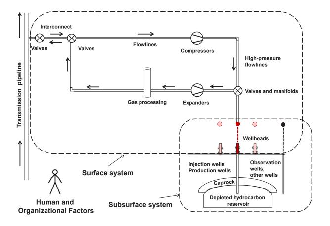
Figure SR-1.2. Simplified schematic of the main components of underground gas storage facilities in California, showing examples of engineered surface components and the wells and geologic features comprising the subsurface system. Human and organizational factors play a critical role in control of both surface and subsurface systems.
