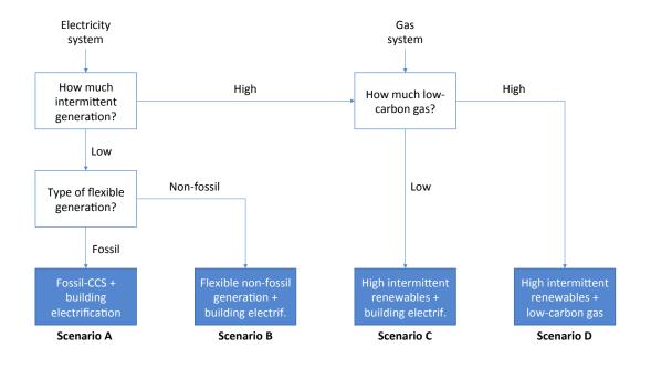
Figure SR-3.4. Logic diagram for 2050 scenario classification.
